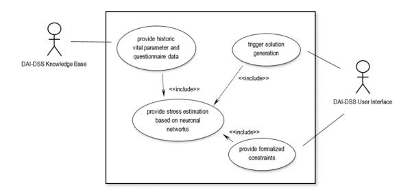
Figure 48 UML-use-case diagram of Operator Stress Estimation Service
