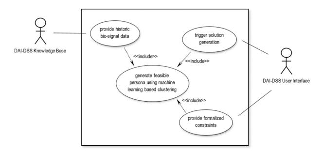
Figure 58 UML Use Case Diagram of Operator Persona Development Service
