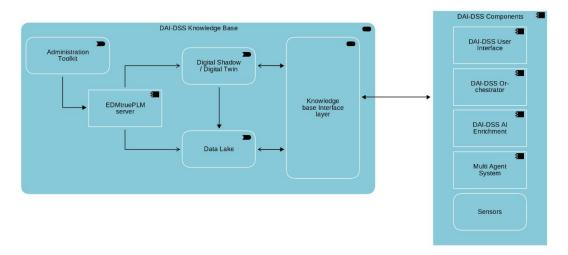
Figure 19 High level architecture of DAI-DSS Knowledge Base
