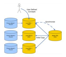
Figure 20 The use of reference data in the PLM Module
