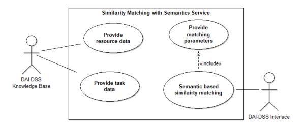
Figure 64 UML Use case diagram for the similarity matching with semantics service
