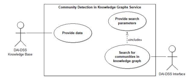
Figure 60 UML Use Case Diagram for the community detection in knowledge graphs service
