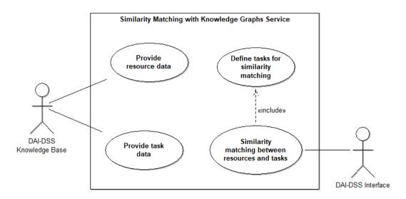
Figure 34 UML Use Case Diagram for the Similarity Matching with Knowledge Graphs service
