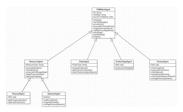
Figure 24 Current agent UML Class Diagram
