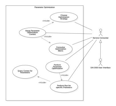
Figure 56 UML-use-case diagram for Parameter optimization service with machine learning
