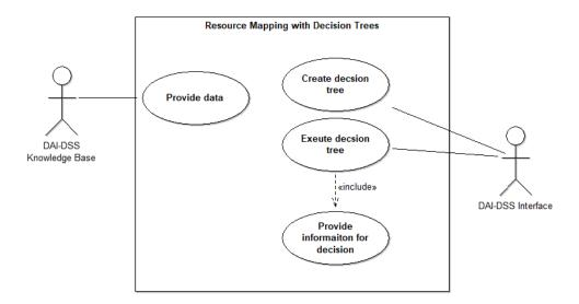
Figure 36 UML Use Case Diagram for the Resource Mapping with Decision Trees Service
