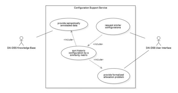
Figure 54 UML Use Case diagram of the Configuration Support Service
