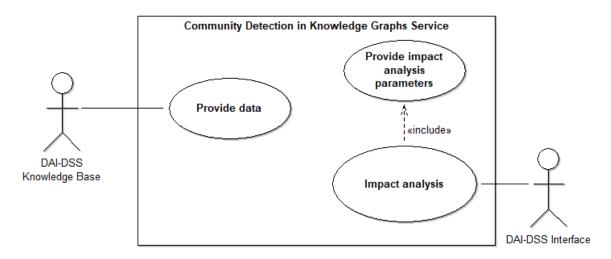
Figure 66 UML Use Case diagram for the impact assessment with knowledge graphs service
