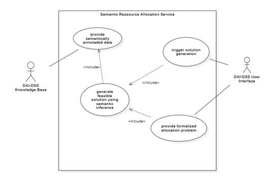
Figure 42 UML Use Case Diagram of the Semantic Resource Allocation Service
