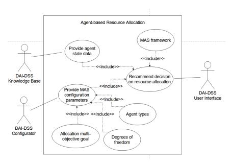
Figure 68 UML Use Case Diagram for Agent-based Resource Allocation
