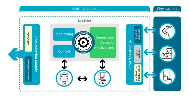
Figure 23 Multi-Agent System: Internal Architecture
