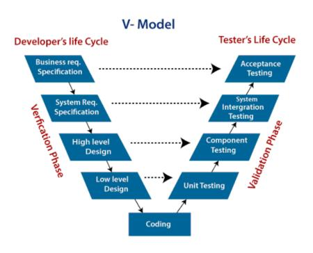
Figure 72 V model Architecture testing
