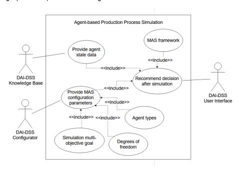
Figure 52 UML Use Case Diagram for Agent-based Production Process Simulation
